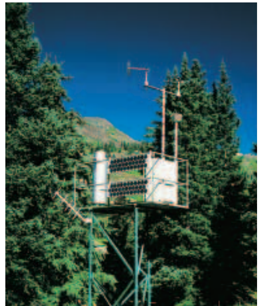
Figure 12-11 This automated weather system measures surface data.
